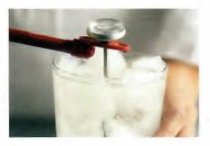
2 Put the thermometer stem or probe into the ice water. Make sure the sensing area is submerged.
