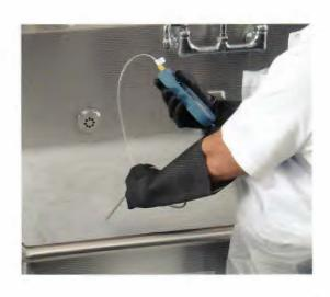
Calibration Thermometers can lose their accuracy. When this happens, the thermometer must be calibrated, or adjusted, to give a correct reading. Make sure your thermometers are accurate by calibrating them regularly. Calibrate thermometers at these times:
