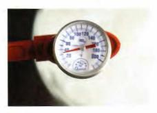
3 Adjust the thermometer so it reads 32°F (0°C).
